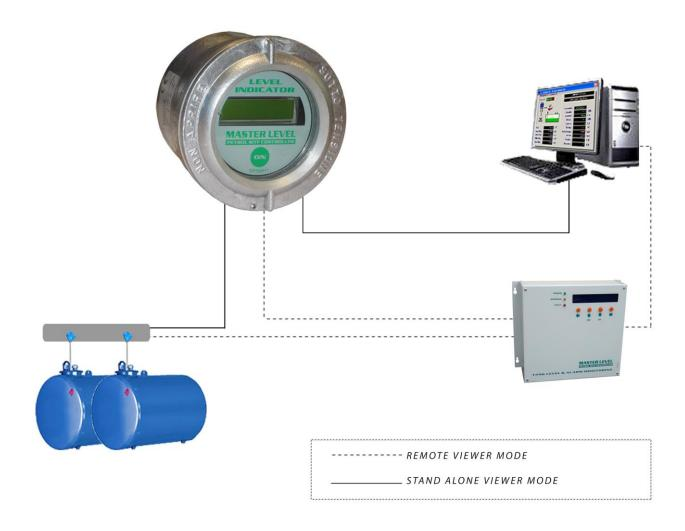
The CPT04111 series device allows the local display of the volume of product stored inside the tanks. It can be used as a <u>Stand Alone local viewer</u> for the connection of 6 AMT series anti-explosion level probes and 2 free output voltage contacts programmable using the MasterLevel Setup or Gsetup software or as a <u>remote viewer</u> connected to MasterLevel or Fafnir series control units Visy-Command.
